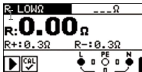
Figure 5.11: Example of  $R_{LOW\Omega}$  result
