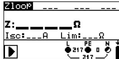
Figure 5.20: Fault loop impedance
