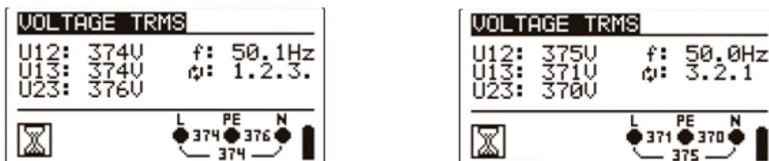
Figure 5.4: Examples of voltage measurement in three-phase system
