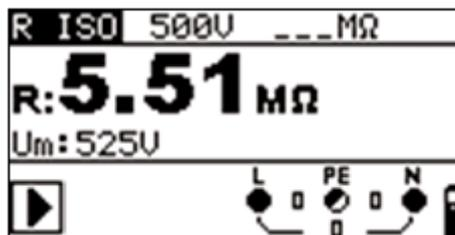
Figure 5.7: Example of insulation resistance measurement result
