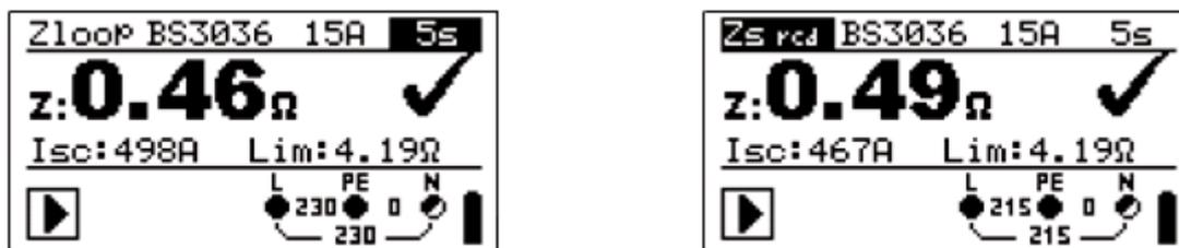
Figure 5.22: Examples of loop impedance measurement result
