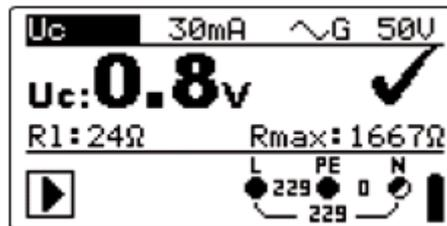
Figure 5.15: Example of contact voltage measurement results
