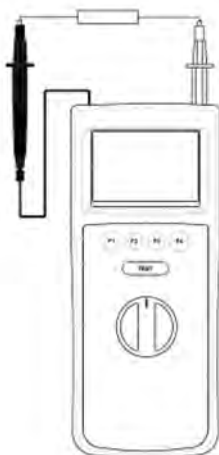
Figure 4 Earth Continuity/Insulation Measurement using Cordless probe
