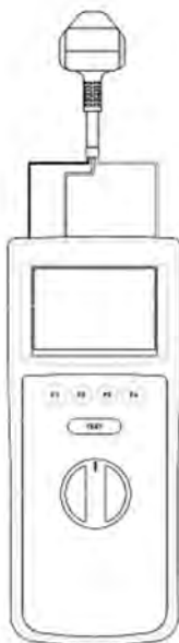
Figure 6 Earth Loop Impedance/Line Impedance/ RCD/ Mains Voltage Measurement
