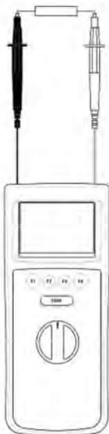
Figure 3 Earth Continuity/Insulation Measurement
