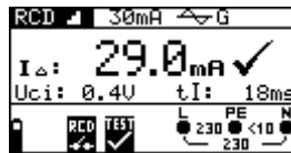
Figure 5.18: Example of trip-out current measurement result
