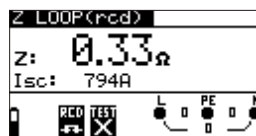
Figure 5.30: Example of fault loop impedance measurement results using trip-lock function
