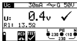
Figure 5.14: Example of contact voltage measurement results
