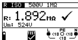
Figure 5.3: Example of insulation resistance measurement results
